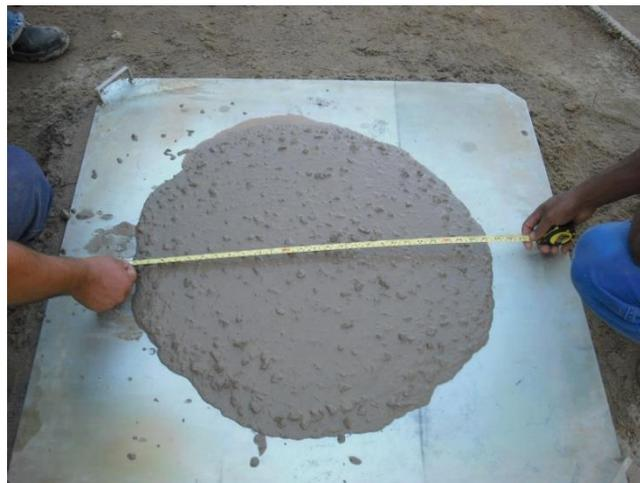
Figure 9. Measurement of concrete flow.
