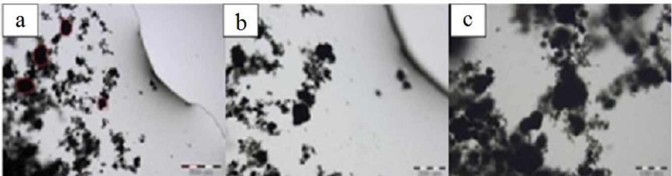
Figure 6. Sample SM 2 - powder CNT dispersed in water and a polycarboxylate admixture (Tec Flow 8000 - at 2%).
