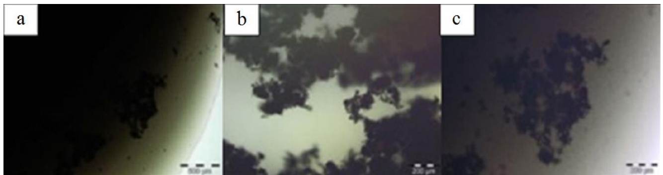
Figure 14. Sample SM 10 - CNT Aquacyl 0301 dispersed in water, with powder CNT and polycarboxylate admixture (Tec Flow 8000 - at 0.5%).
