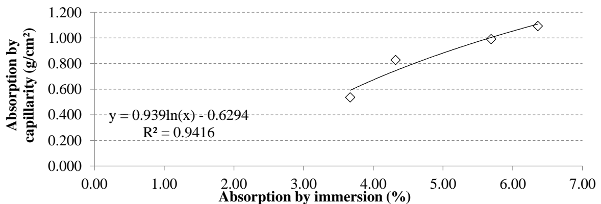
Figure 10. Correlation between water absorptions by immersion and by capillarity.
