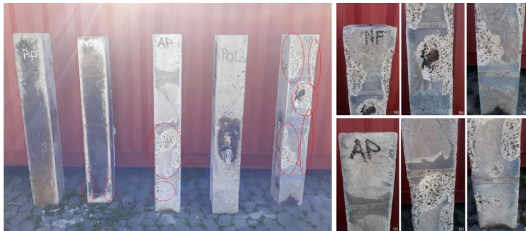
Fig. 10. Columns after being subjected to the fire and focus in NF and AP post fire, showing the top (a), center (b) and base (c).
