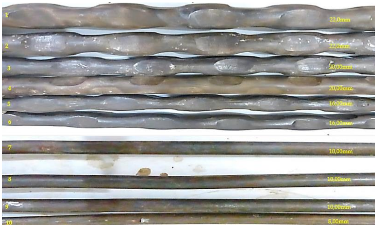
Figure 14. Classification of steel samples according to his gauge (Source: Arcelor Mittal)
