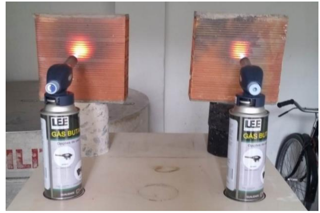
Figure 7. Blocks without passive protection.
