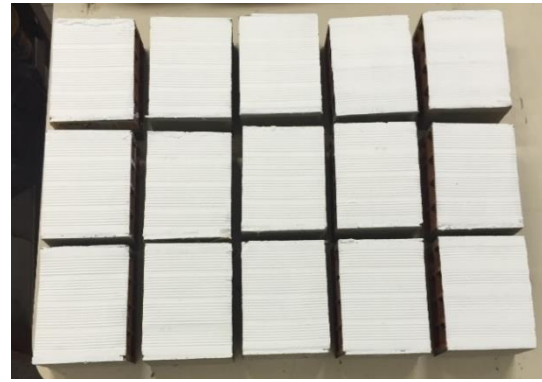
Figure 4. Application of intumescent paint.
