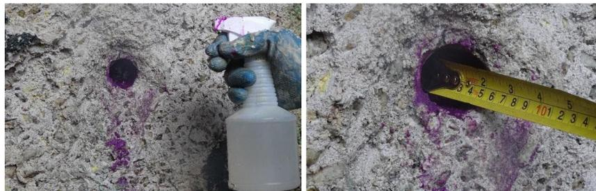
Figure 4: wet-well’s wall - alkaline concrete
