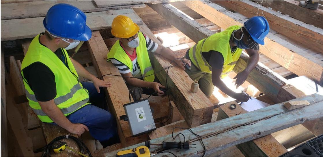
Figure 9. Application of UPV tests on wooden beams
