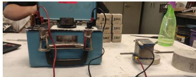
Figure 4. Nilsson resistivity apparatus.
