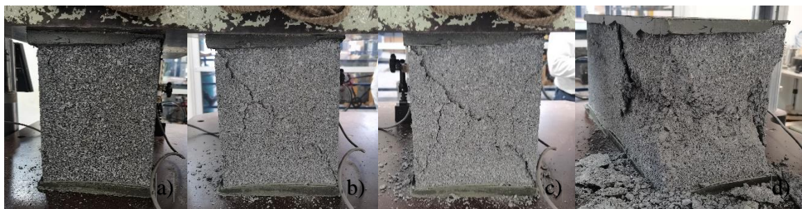
Figure 6. Stages of the cracking process of the HCB capping over gross area: a) Cracking begin at the corners of the block, b) and c) development of cracks towards the center of the block faces, d) detachment of segments of the material. Sources: Own elaboration.
