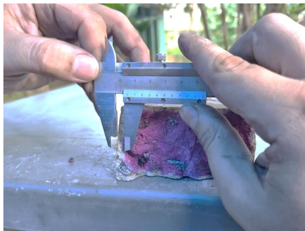
Figure 7. Measurement of the carbonated area
