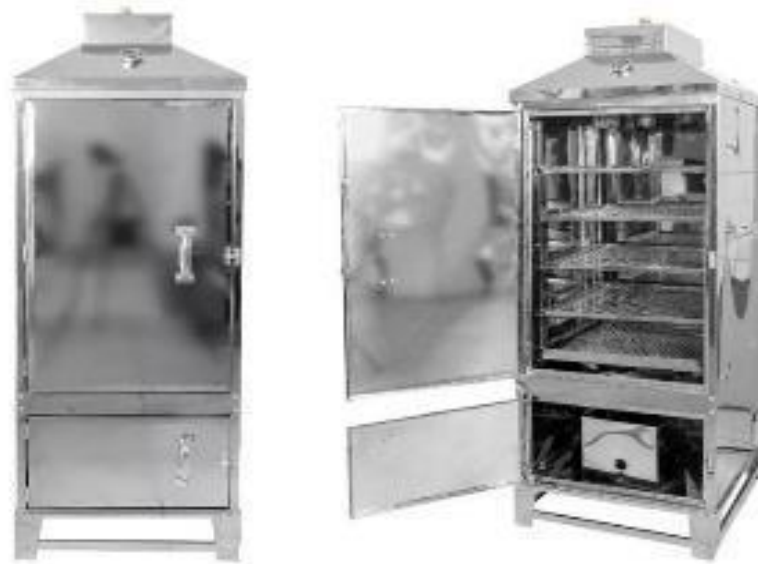
Figure 2. Smoker used as a covering for burning the specimens.
