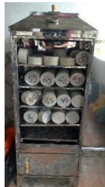
Figures 4 and 5. Left: Materials for burning inside the casing. Right: Test specimens arranged inside the casing, with each trace arranged at one level of the casing.
