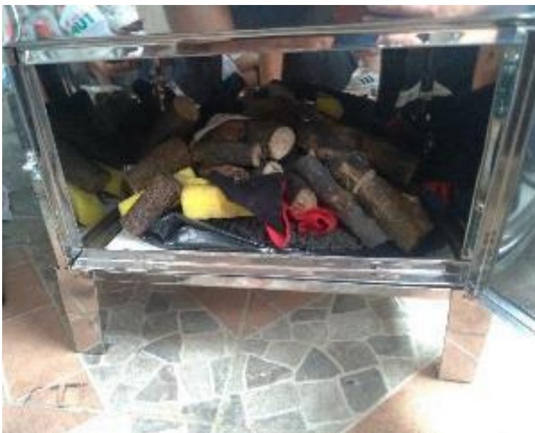
Figures 4 and 5. Left: Materials for burning inside the casing. Right: Test specimens arranged inside the casing, with each trace arranged at one level of the casing.
