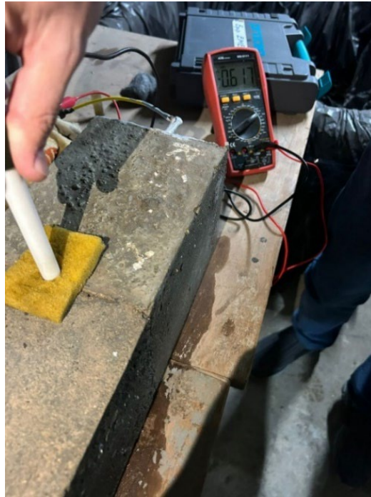
Figure 5. Equipment for conducting corrosion potential ( E_{corr} ) tests.
